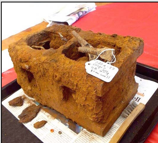
This unidentified electrical device had field coils, and once had two armatures.
