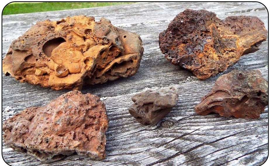
Formations of slag of different types from the beach area. These are residue from the bloomery, deposited here before 1811.
