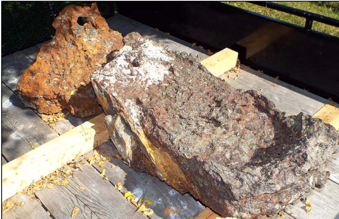
Pure Smelted Iron from the bottom of the furnace.
